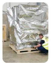
The 3D barrier bag is sealed to the base sheet with a hand held heat sealer.
