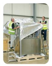
The base sheet is laid on the case base. Desiccant is added & the bag is placed over the machine.
