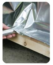
A small gap is left at the end of the seal, and the air is evacuated from the bag with a shop vac.
